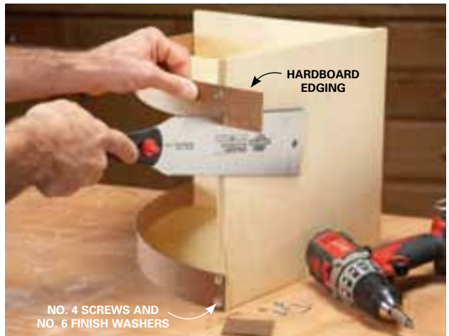
1 Install the edging, then trim it. Cut the hardboard edging a few inches too long, fasten it with screws and slice off the excess with a fine-tooth saw. Finish washers give the screws a neater look.
