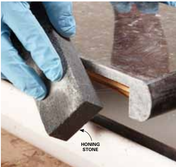
3 Rub cut edges with a honing stone to bevel the edge slightly. Rub in a circular motion to avoid wearing a groove in the stone.
