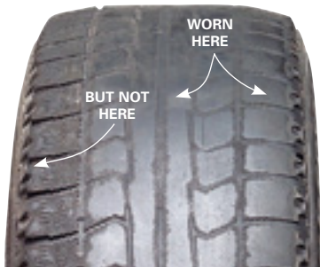
Uneven tread wear signals alignment problems
